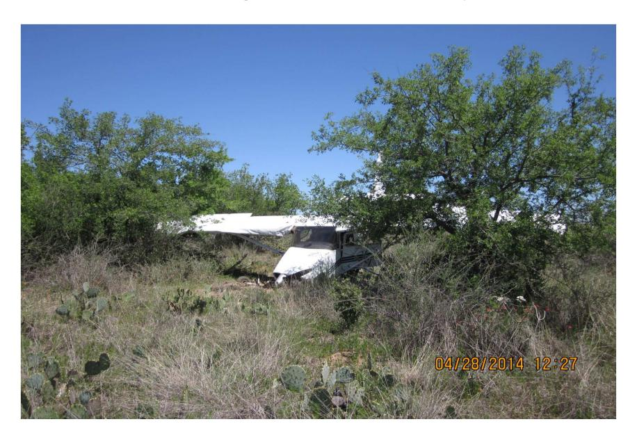
Stinson – Mooney M20TN Pilot was doing touch and goes on runway 14 but was lined up for 9, when questioned by ATC he turned to base for 14. Pilot claims the engine did not respond to the throttle resulted in a stall and off airport landing. No Injuries, 44709 pending
