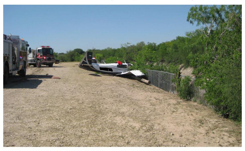
Pleasanton, TX. N167T With 5 PAX the 5000 hr. ATP pilot attempted downwind landing, going to fast executed a go around. Stalled aircraft impacted ground left of runway. All PAX sustained minor injuries. 44709
