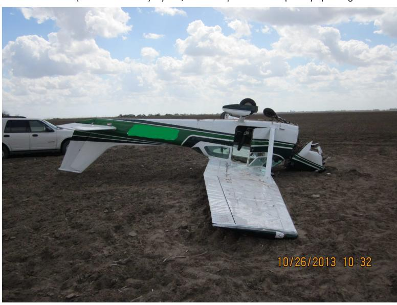
PA28-140 Engine lost power on takeoff. Restricted induction airflow due to the wrong induction air tubing installed, and restricted exhaust flow. The pilot received serious injuries. Pilot will be counseled on engine out procedures.
