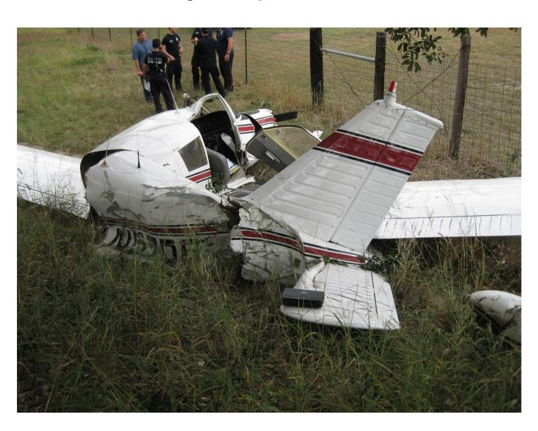
Leakey, TX. - Zenith 601XL Canopy opened on takeoff distracting the pilot, resulting in steep angle and hard landing. (1 serious injury)
