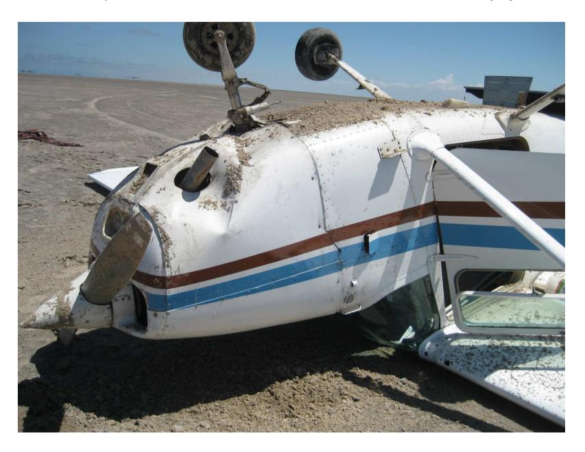
Cessna 172 -Llano, TX. Lost power on takeoff. Engine analytical tear down is pending. 3 people onboard – no injuries.
