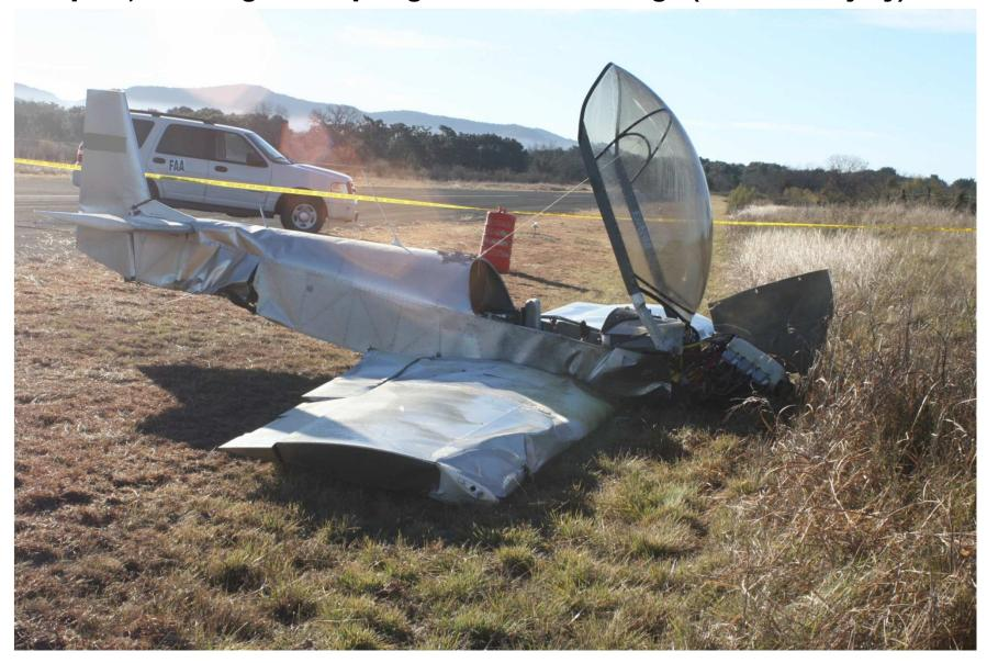
Cotula, TX. Pilot Error –Cessna 172 hard landing and loss of control. Flight instruction flight. Loss of control on Ldg. CFI took controls too late. 1 minor injury, Pilot 44709
