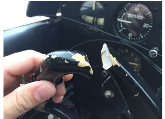
Valerie's 182 yoke showing the point of failure.
