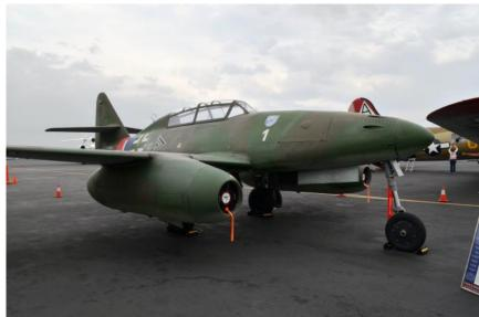
The replica Messerschmitt Me 262 twin jet fighter, is one of three of which have been built. Two are in the U. S. and one is in Germany. The airframe and aerodynamics have been duplicated to exacting standards. The engines have, of necessity, been upgraded. The design incorporates many features seen today in modern aircraft., one of which is swept wing technology.
